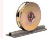
2) Cantilevered Gates: the cantilevered gate runs across the gate opening without actually touching the surface. Thus it is ideal for uneven or slightly sloping ground. The gate includes an inverted 'U' shaped lower beam that runs over and is balanced between two permanently fixed guide support rollers. The rollers are secured to a large counterweight concrete foundation.
