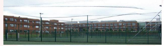
Roof netting is typically suspended high above the court on one or more high-tensile linewires, and gently sags down either side to the perimeter fence. The top linewires are tensioned between steel straining posts, set into concrete bases at either end of the court.
