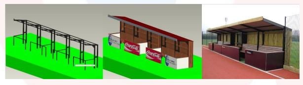
Typically they are 12 metres long comprising three compartments: one each side for the home and away teams with 5 metres of timber bench seating and baggage racks; plus a 2 metre gated central area for scoring/umpire etc. An inner central door gives access to the rear (for ball retrieval).
